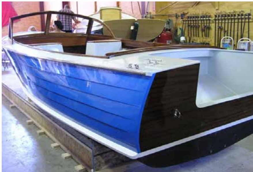
The second-year students also finished the commissioned 18' Tad Roberts Runabout. The paint job and finish work is striking and looks as good as any professional job I've seen. The owner is quite pleased with the result.
