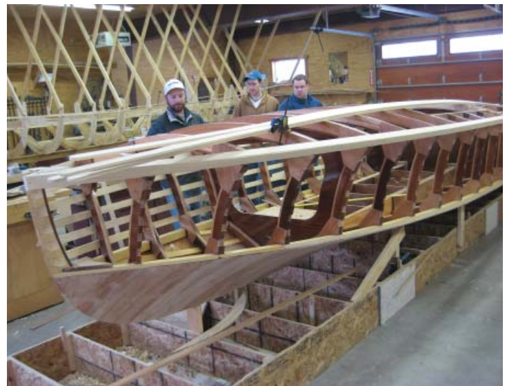
L to R: 2nd-year students Nic, Adam, and Gus attaching the battens on Hacker Dash Two.
